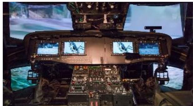
Figure 2. Cockpit with eye tracking cameras in place.
